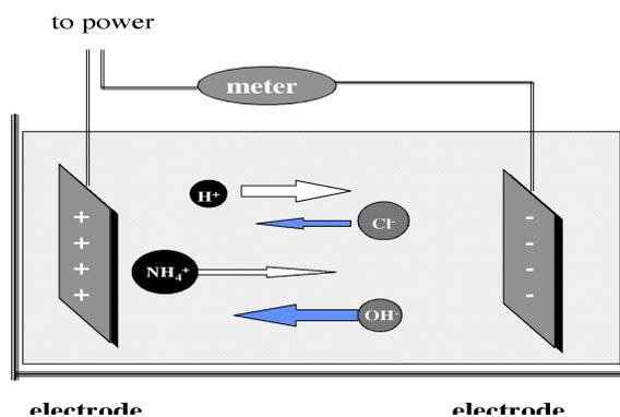
**Figure 1.** Schematic of a simple conductivity measurement system.
