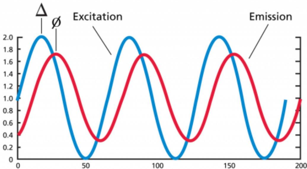
Each probe has a slightly different response to oxygen concentration, so prior to use it must be calibrated using known levels of oxygen. Once the phase shift is measured, it can be related to the oxygen concentration or partial pressure using the Stern-Volmer equation. If pressure and temperature cannot be controlled and kept constant from calibration to measurement, they must also be factored into the calculations, and a multi-point calibration must be used.
