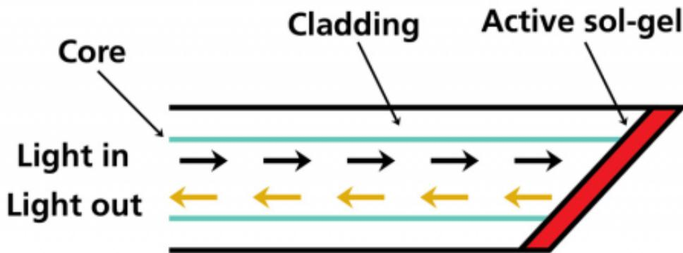
A more subtle effect of fluorescence quenching is that the average fluorescence lifetime of the indicator material decreases as oxygen concentration increases. By pulsing the excitation LED and looking at when maximum fluorescence is emitted relative to those pulses (the phase shift), the average fluorescent lifetime can be determined. This method is called phase-sensitive detection. This is the method used by all OOI NeoFox systems.
