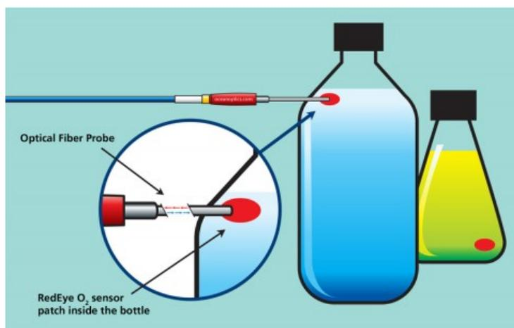
OOI particular oxygen sensors use a blue LED for excitation at 450 nm, transmitted to the sensor material using a fiber optic probe. Fluorescence at visible wavelengths is collected back through the same probe and routed to an avalanche photodiode for detection.
