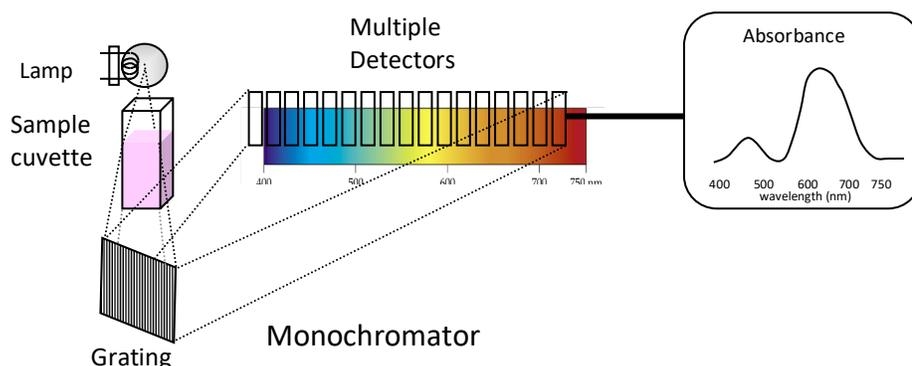
Figure 2: A spectrophotometer based on a multi-wavelength detector (PDA).
