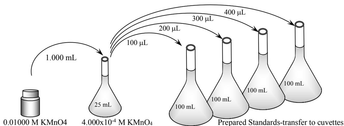
Figure 5: Successive dilutions scheme for the preparation of 0.709-0.284 mg/L equivalent  $\text{Cl}_2$  standards from 0.01000 M  $\text{KMnO}_4$ .
