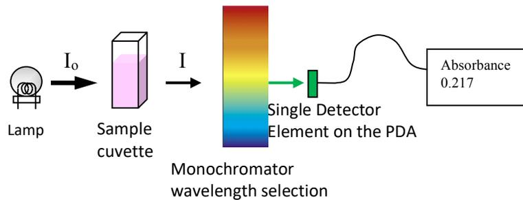
Figure 3: The intensity falling on the sample is  $I_0$  and the intensity after absorption by the sample is  $I$ . The intensities are measured separately at each wavelength.
