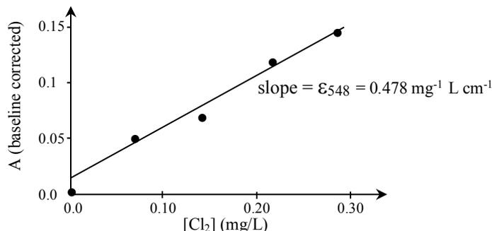
Figure 4: The calibration curve for DPD with concentrations expressed as mg/L Cl<sub>2</sub>.
