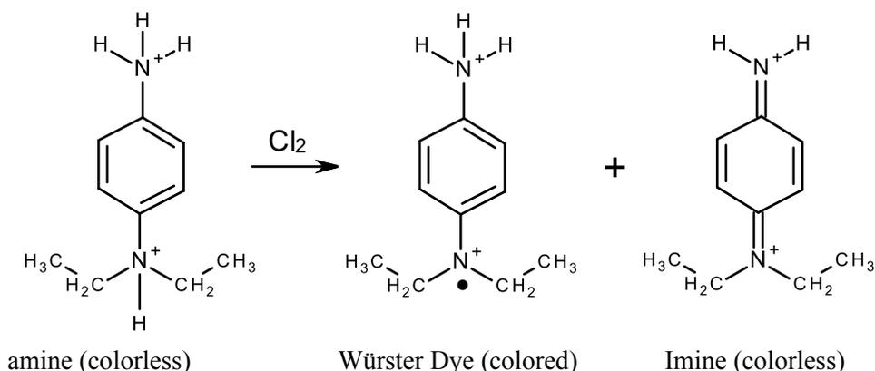
Figure 1: DPD (N, N-diethyl-p-phenylenediamine) is oxidized to a colored product by  $\text{Cl}_2$ .
