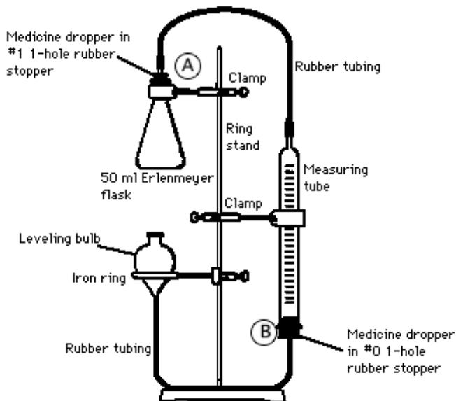
**Figure 1.** Apparatus for measuring the gas produced from the reaction of a  $NaCl/NaNO_2$  mixture with sulfamic acid. An inverted buret is used as the measuring tube.
